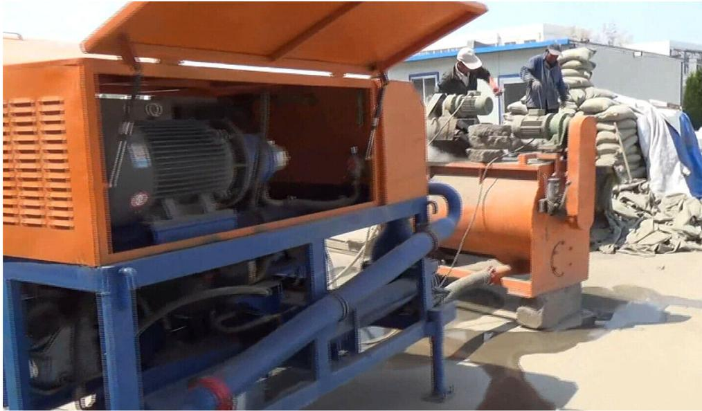
**GF30 cement foam machine Technical data:**
