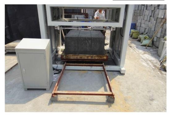
It is specially used to cut various foam concrete blocks. Easy operation, high efficiency. The block size between 100-200-300-400-500-600-700-800-900-1000-1100-1200mm could be adjusted willfully.
