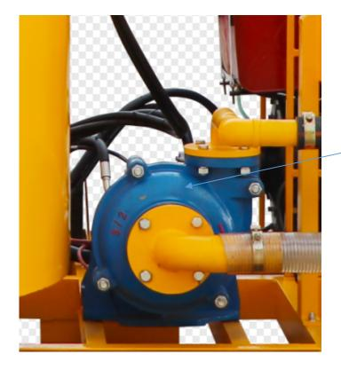
Heavy-duty slurry pump for recirculating and discharging
