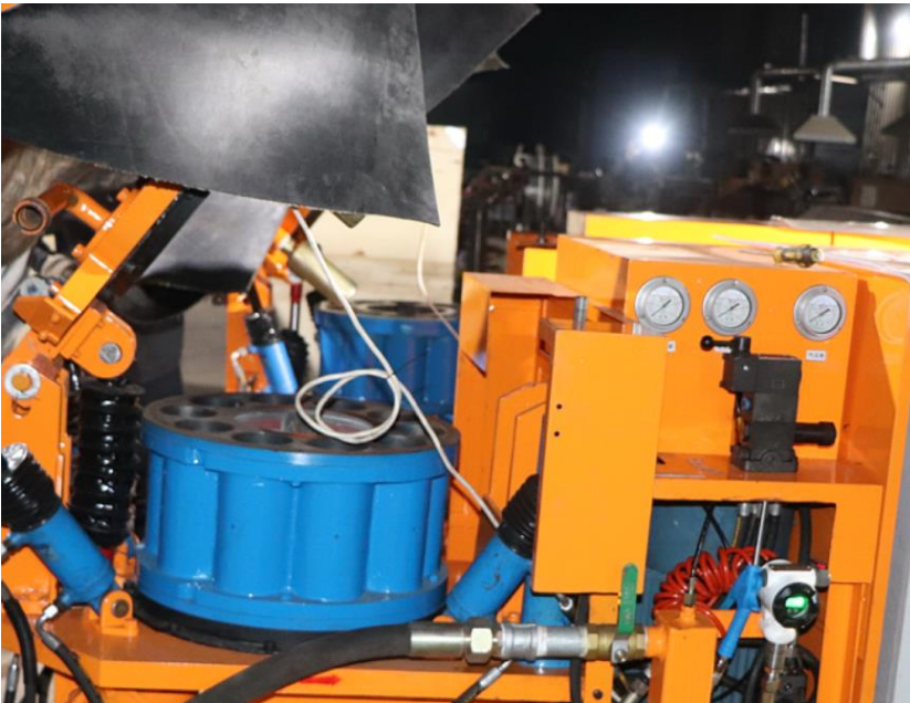
Hydraulic lift the rotor
